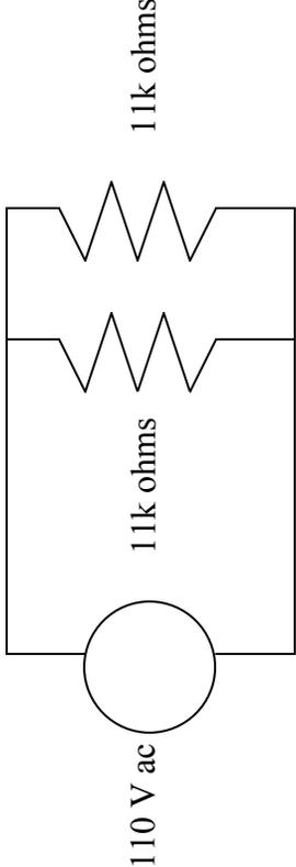
Calculate the voltage across each resistor. What is the equivalent resistance value of the two resistors in series?
