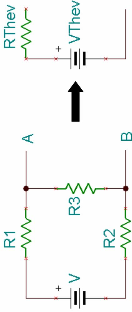
Any circuit of resistors and sources can be reduced to a single source and resistor – the Thevenin's equivalent.
