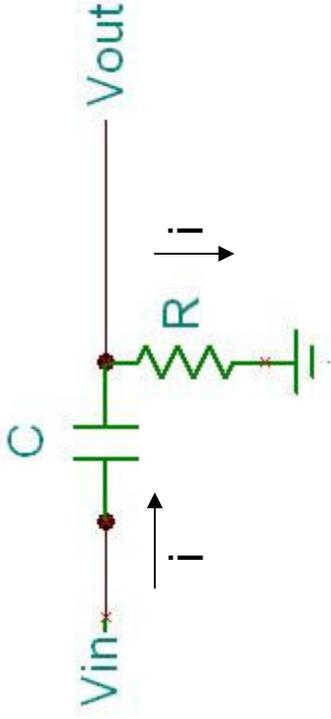
$$i = C d(V_{IN} - V_{OUT})/dt = V_{OUT}/R$$
