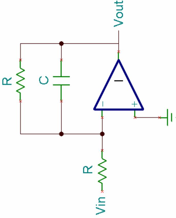
Recall impedance, inverting amplifier.
