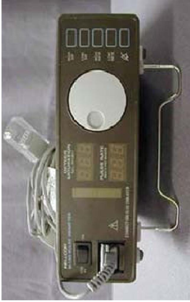
The pulse oximeter is a spectrophotometric device that detects and calculates the differential absorption of light by oxygenated and reduced hemoglobin to get  $sO_2$ . A light source and a photodetector are contained within an ear or finger probe for easy application.
